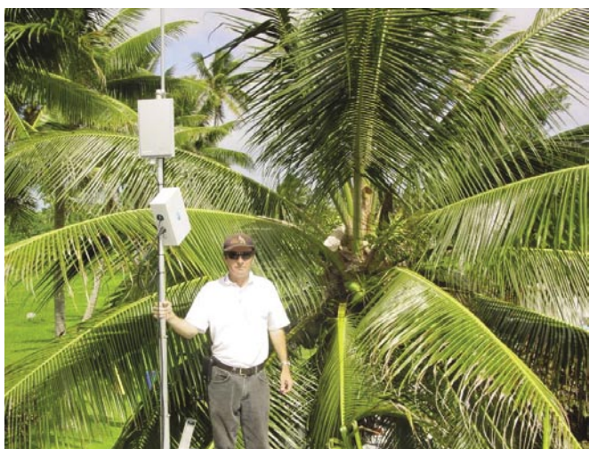
St. Clair with the Trango Access Point and antenna units used for WiFi systems serving Niue's outer villages.
